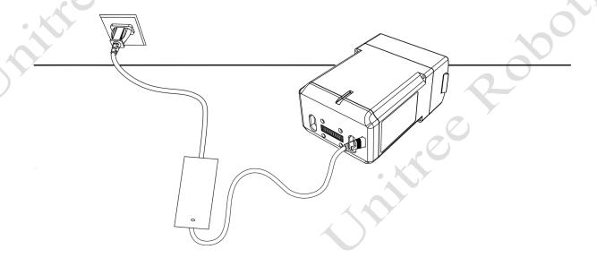
Charging battery indicator: The battery LED light shows the current battery while charging.
