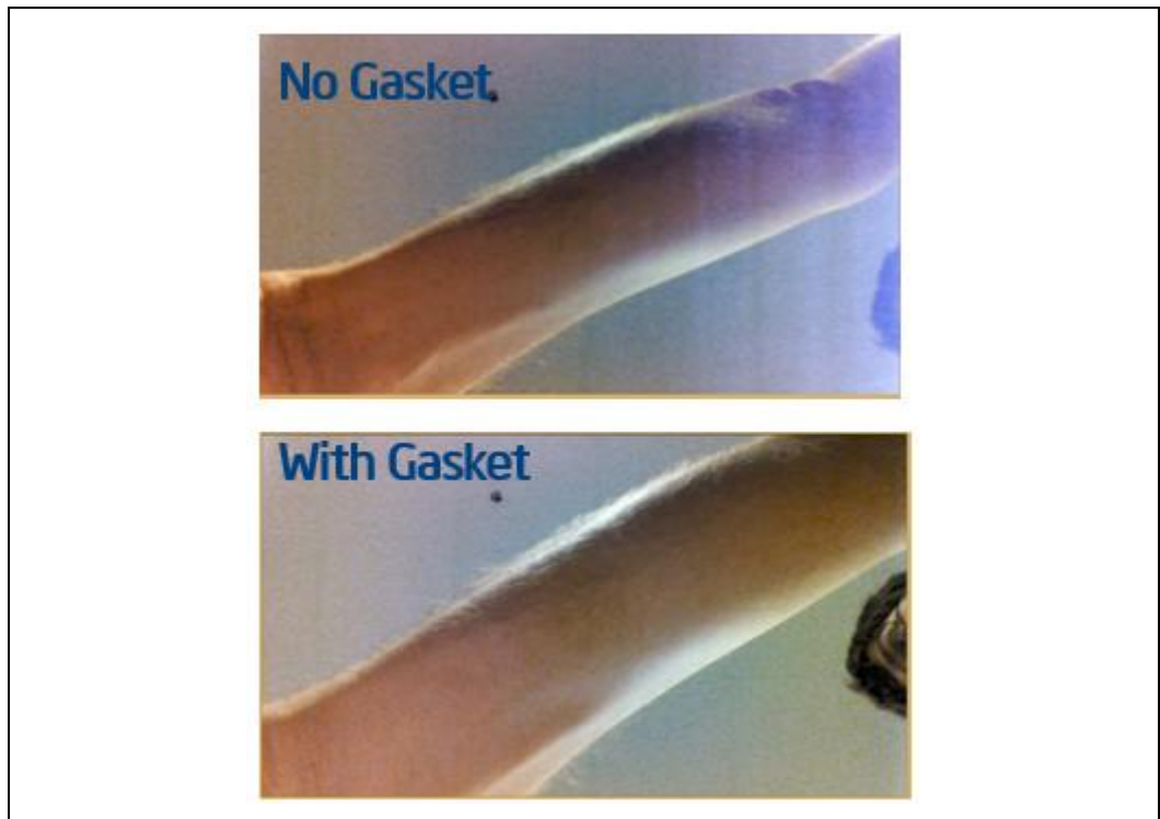
Figure 7-18. Example of Light Leakage Effects
