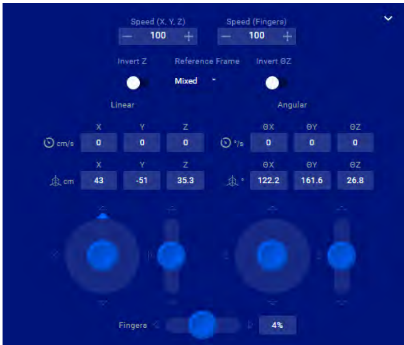
Figure 28: Pose joystick panel
