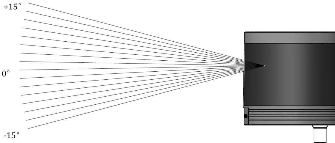
Figure 15 RS-Helios-16P Vertical Angles
