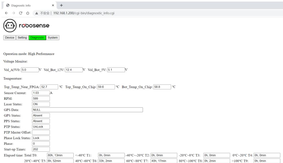
Figure A-3 Diagnostic Screen at the Web Interface
