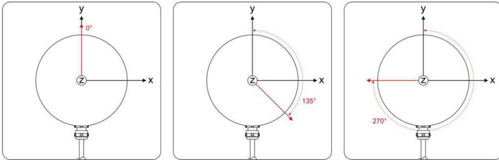
Figure 8 RS-Helios-16P Different Phase Settings
