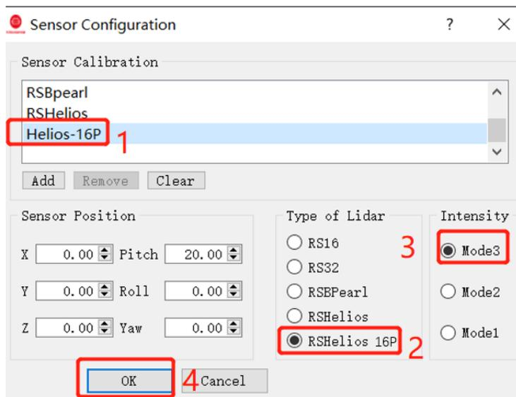
Figure C-2 Select RS-Helios-16P Parameter Configuration File
