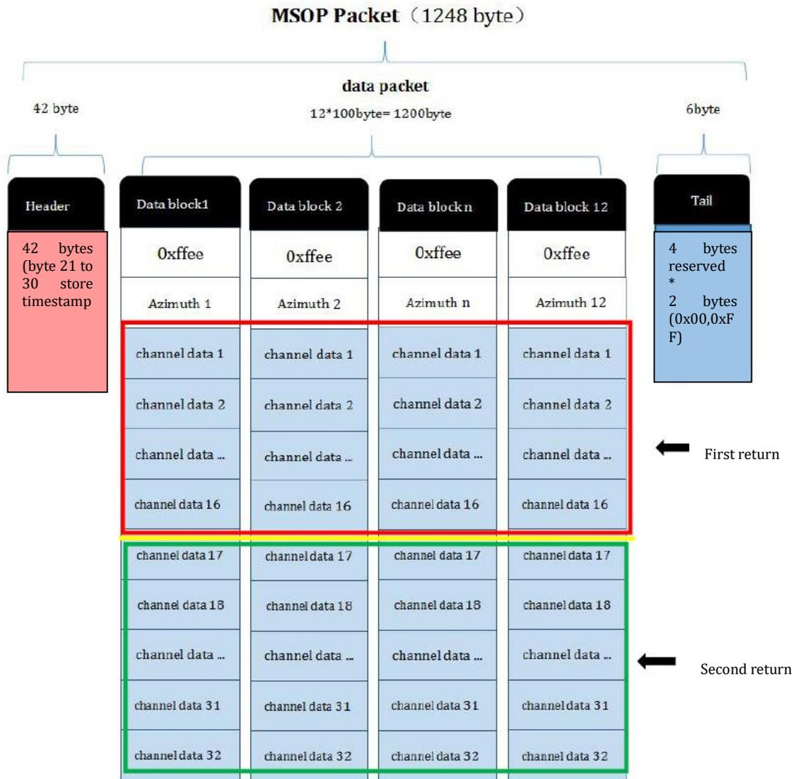
Figure 13 MSOP Packet Definition of Dual Return Data
