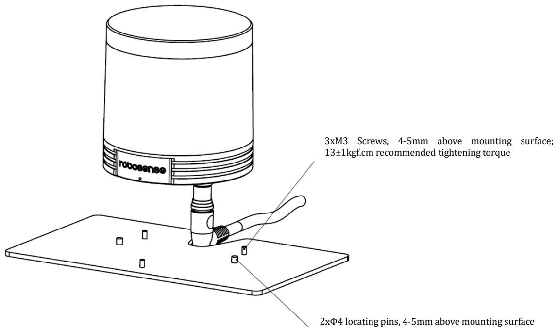
Figure 4 LiDAR Mounting Details
