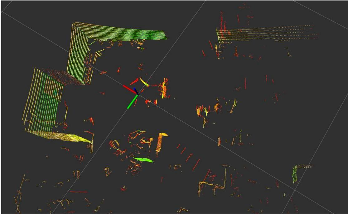
Figure D-1 rviz displays RS-Helios-16P point cloud data
