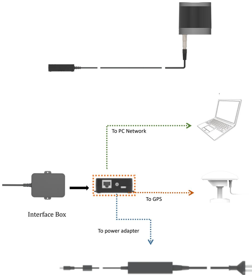
Figure 6 Interface Box Connection
