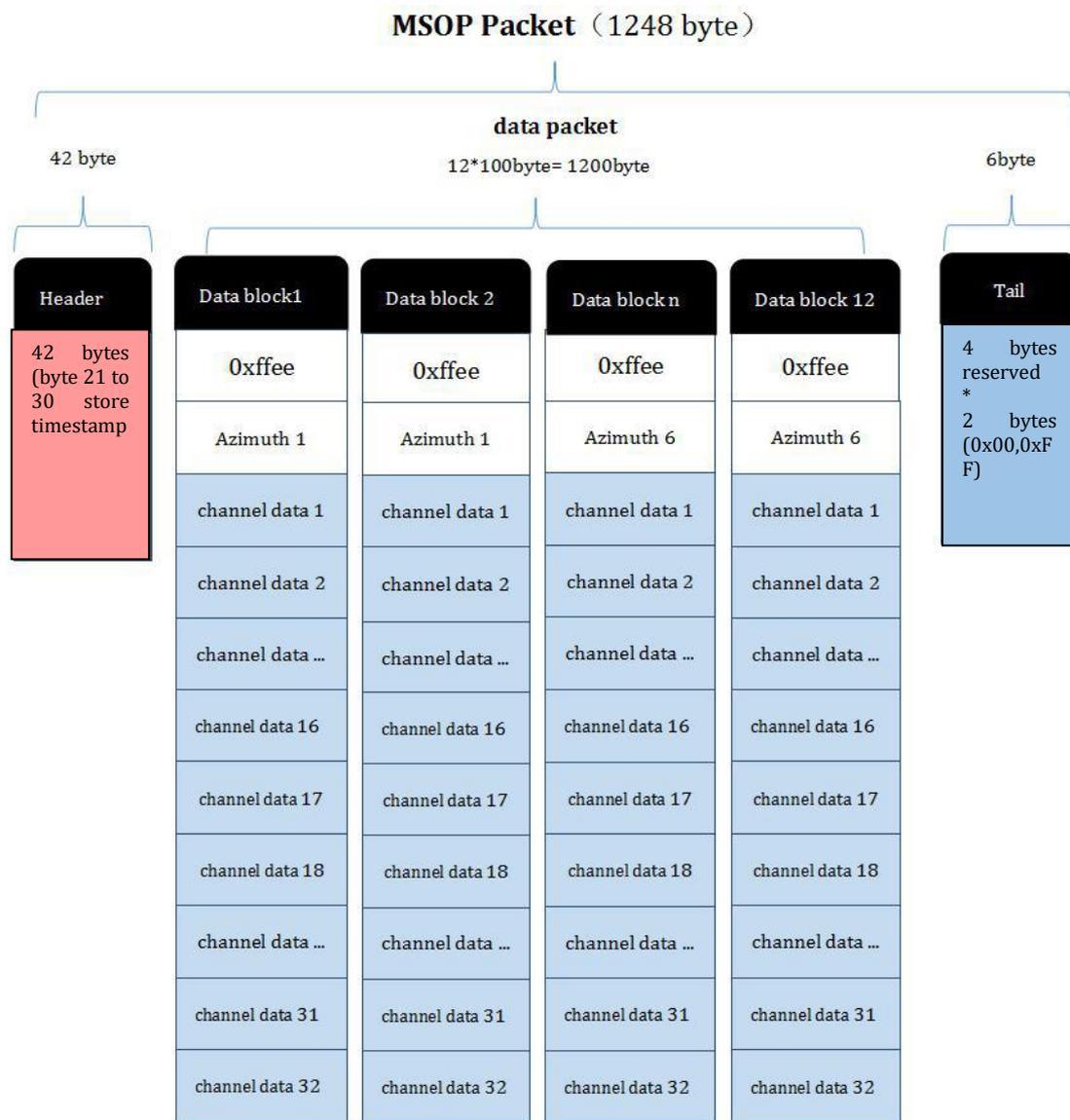
Figure 12 MSOP Packet Definition of Single Return Data
