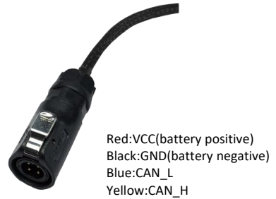
Figure 3.2 Schematic diagram of aviation plug male connector
