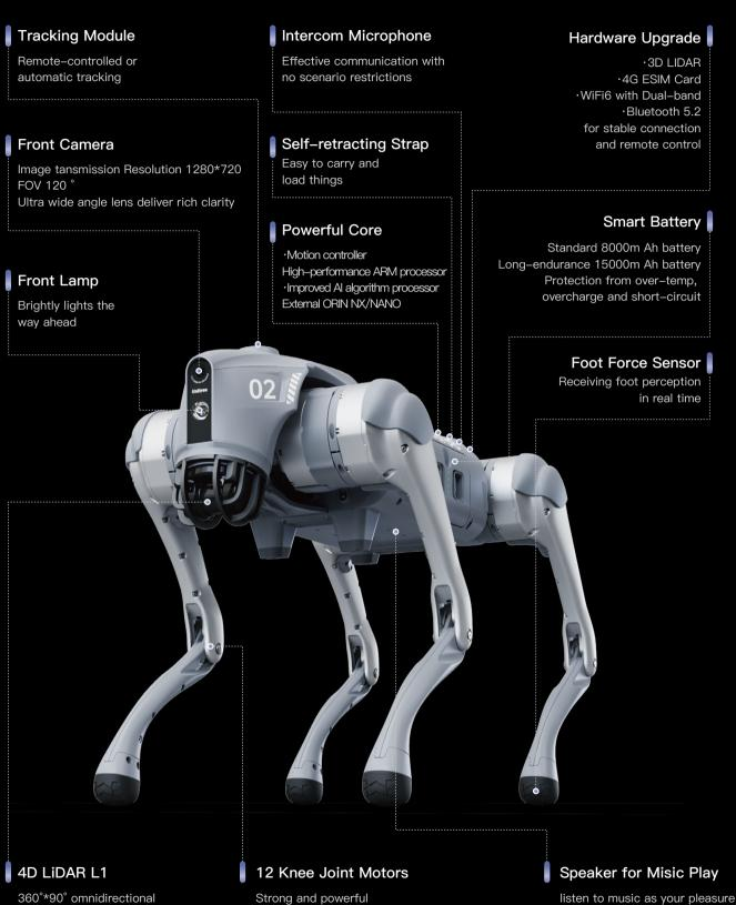
ultra-wide-angle scanning allows automatic avoidance with small blind spot and stable operation
