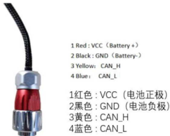
Figure 3.1 Schematic diagram of aviation plug
