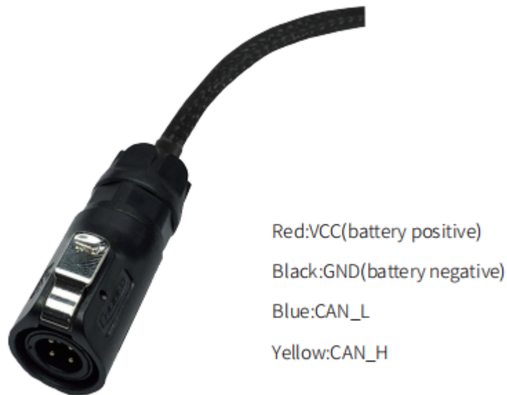
Figure 3.2 Schematic diagram of aviation plug male connector
