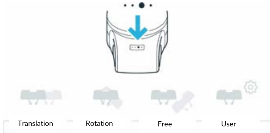
Fig. 13.21: Overview of switching between Hand-Guiding-Modes
