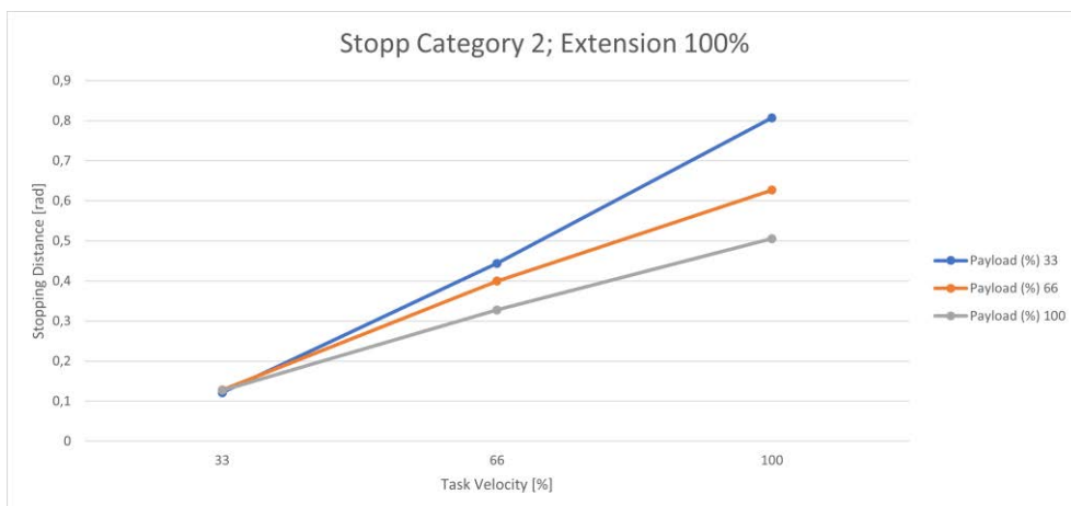
Fig. 17.28: Distance; Stopp Cat 2; Joint 1 100%
