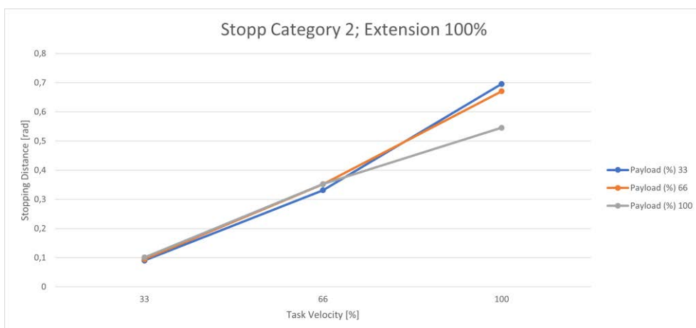
Fig. 17.40: Distance; Stopp Cat 2; Joint 3 100%
