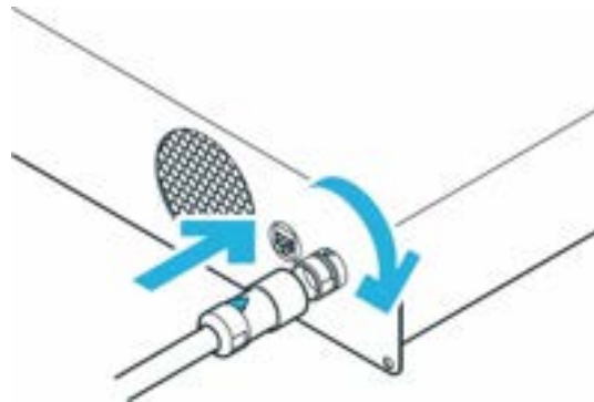
Fig. 10.22: connection of connecting cable to the control
