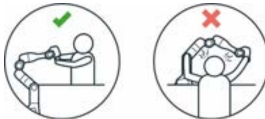
Fig. 10.29: Distance to arm bumping the head
