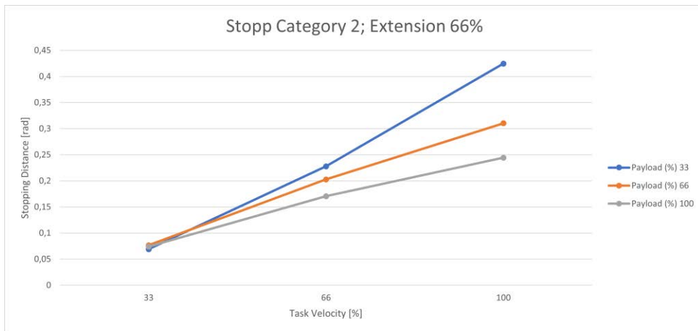
Fig. 17.42: Distance; Stopp Cat 2; Joint 4 66%
