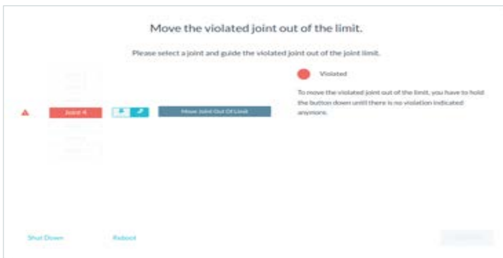
Fig. 13.27: Message with display of the faulty joint
