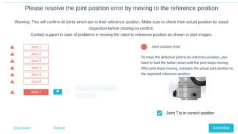
Fig. 13.38: Confirm the complete recovery
