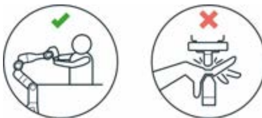
Fig. 10.31: Distance to arm Squeezing the hand
