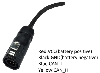
Figure 3.2 Schematic diagram of aviation plug male connector
