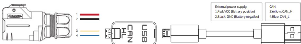
Figure 3.4 CAN Connection Diagram
