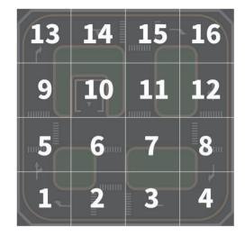
Splice the bottom plate in the order of the bottom plate stickers and referring to the bottom plan; the numbered stickers are unified on the upper right corner of the back of the bottom plate.
