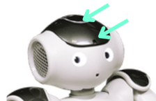
Place your hand on NAO's forehead, covering her camera, and press the first button.
