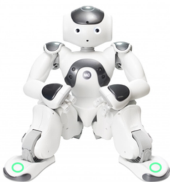
Green feet LEDs = NAO Activities (AI) mode activated
