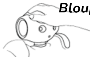
Place your hand on NAO's forehead, covering her camera, and press the first button.
