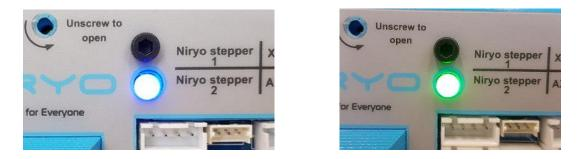
(i) Once the LED is blue or green, it means that the robot is fully started and you can start using it.
