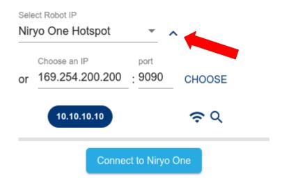
Write "169.254.200.200" (static IP) and click on "Choose" to select the IP address. Note that selecting the IP address just means that this IP will be used by Niryo One Studio, it does not mean that you are connected to the robot.
