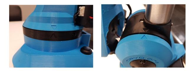
Make sure that the mechanical parts are correctly lined up (+/- a few degrees), if the difference is too big you'll get an unwanted offset on some axis.
