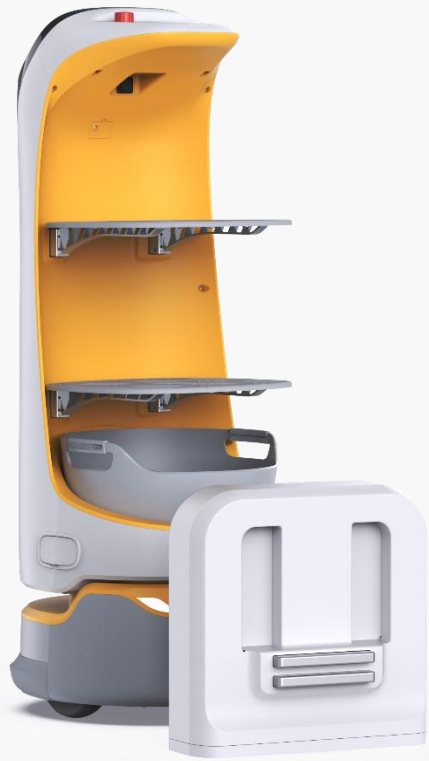
Station de charge
