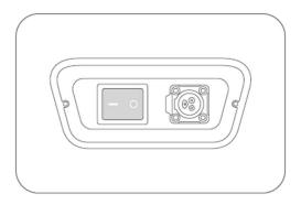
Step 2 Move the robot to the startup location. Press and hold the power switch for 1 second, and the light strip on the top of the robot will turn blue, indicating that the robot has been successfully powered on.
