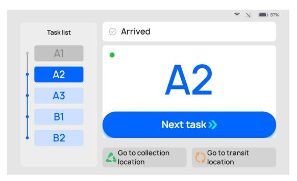
Step 3 When robot reaches its destination, the operator can put items on robot's trays and tap "Next task". And then, the robot will then begin executing its destination.
