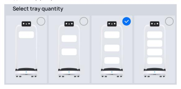
The number of trays can be selected according to the actual number of pallets actually assembled by the current robot. The selection range is 1 to 4. After modification, the number of trays in the robot schematic diagram on the left will be changed accordingly on the home page of each mode.
