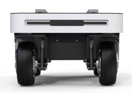
RANGER mini 2.0 adopts a four-wheel independent suspension system with a load capacity of 80 kg, which can effectively improve the robot's maneuverability, pass-ability, and safety. It has the ability to adapt to difficult fields of various industry scenes, with an over 15° slope and 80 mm over ridge.
