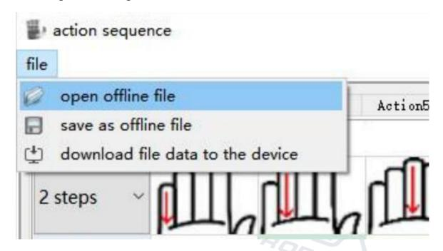
"Open off-line files": This option can be used to open an action sequence data file and display the data in the action sequence data area of the software.
