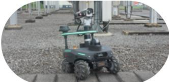
**Larger chassis and all-terrain wheels**, capable of overcoming obstacles up to 14 cm, improving mobility and stability on uneven surfaces.
