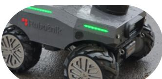
**IP55 protection**, ensuring resistance against dust, rain, and harsh environmental conditions.
