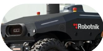
**Native integration of speakers, LED lights, and microphone**, enhancing communication, visibility and interaction during operations.
