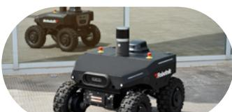
**Extended operational autonomy**, with a 29A battery that significantly increases the robot's working time without interruptions.
