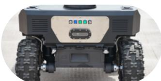
**Easy Swap battery**, removable and easily replaceable by the user. Allows the use of additional batteries to maintain continuous operation without charging downtime; the robot can also be transported without the battery to simplify logistics.
