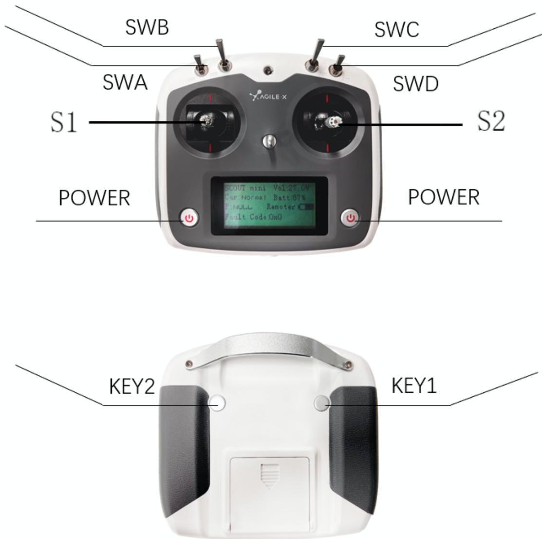
Figure 2.7 Schematic Diagram of Buttons on FS RC transmitter
