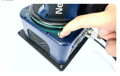
When your robot is switched on, you can run an initial test by launching the demo programme by pressing the button on the base of the robot.
