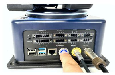
You can switch on your robot by pressing the power button and waiting for the LED ring to light up, turn blue and the robot start-up sound starts. If it's your first start-up, it may take a few minutes.
