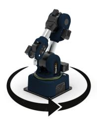
Place the robot on a flat surface with plenty of room around it to avoid any collisions with its surroundings. You can also attach it to its stand using the holes in the base.
