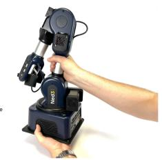
Keep a good posture when moving the robot to avoid any damage
