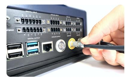
Connect the emergency stop in the same way and make sure that the emergency stop button is not engaged before starting your robot.
