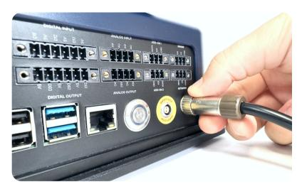
Connect the power supply to the robot's backpanel and make sure that the safety catch is engaged by turning it to prevent the risk of it being ripped off.
