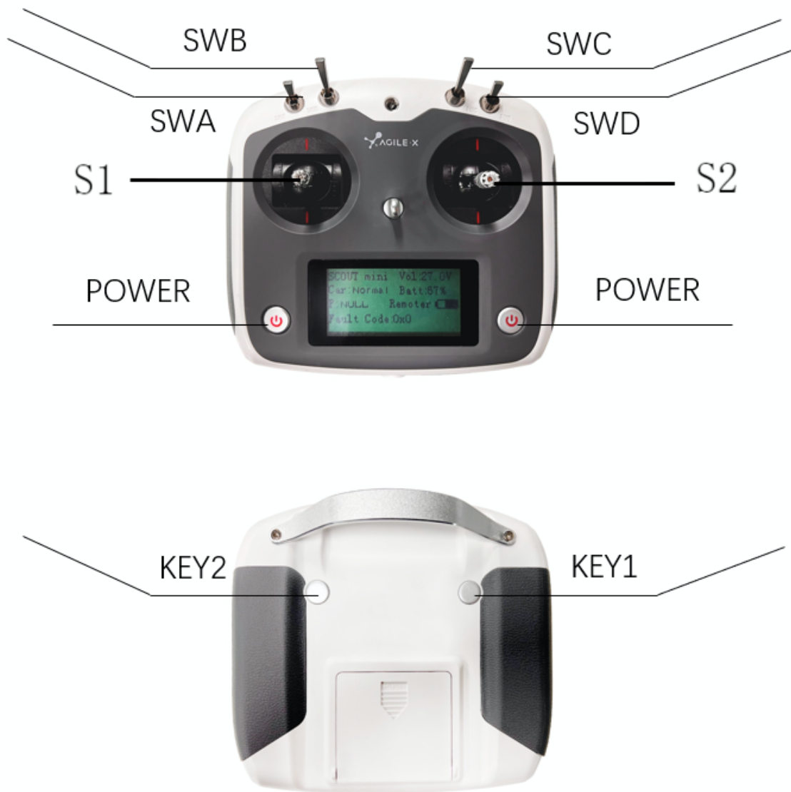
Figure 2.6 Schematic Diagram of Buttons on FS RC transmitter
