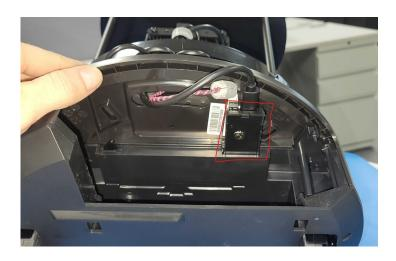
If the cable is correctly connected, you should see a green LED light up on the Rpi card.
