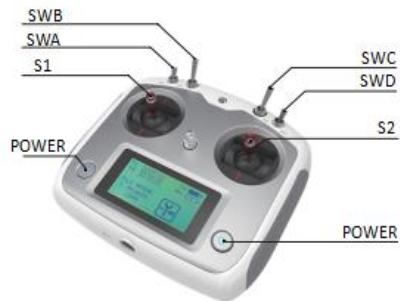
Figure 2.3 Schematic Diagram of Buttons on FS RC transmitter
