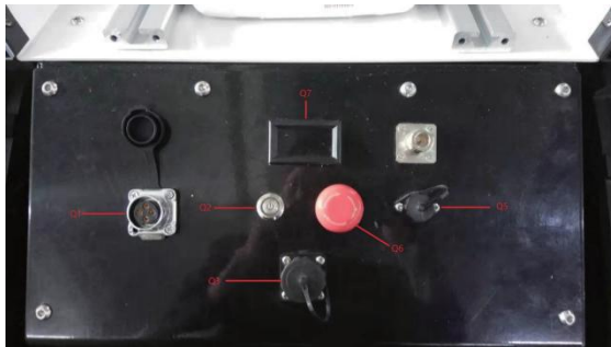
Figure 2-1 Tail electrical interface
