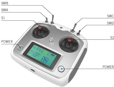
Figure 2.3 Schematic diagram of FS remote control buttons
