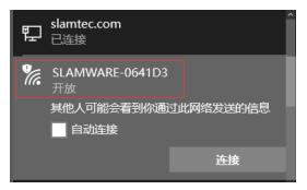
Please connect to the above SLAMWARE- XXXXXX network (you can also connect SLAMTEC MAPPER to PC via Ethernet cable. Please set the network mode as DHCP client).
