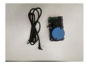
Please put the SLAMTEC MAPPER on a flat surface, and connect to 5V power source with the enclosed power cable.
