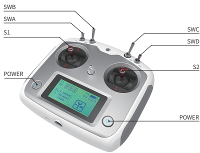
Figure 2.6 Schematic Diagram of Buttons on FS RC transmitter
