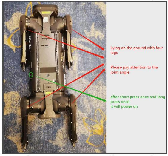
When robot power on, it will enter the normal mode directly.
