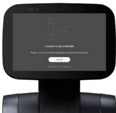
temi is alerting that it has lost its map and requests to be placed on the home base. The home base is the map's anchor point. After placing temi on its home base, the following notification should pop up: (NOTE: This can be modified in the settings! Refer to pg. 24 to learn how)
