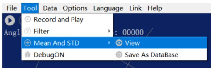
FIG 14 YDLIDAR G2 DISPLAY MEAN AND STANDARD DEVIATION
